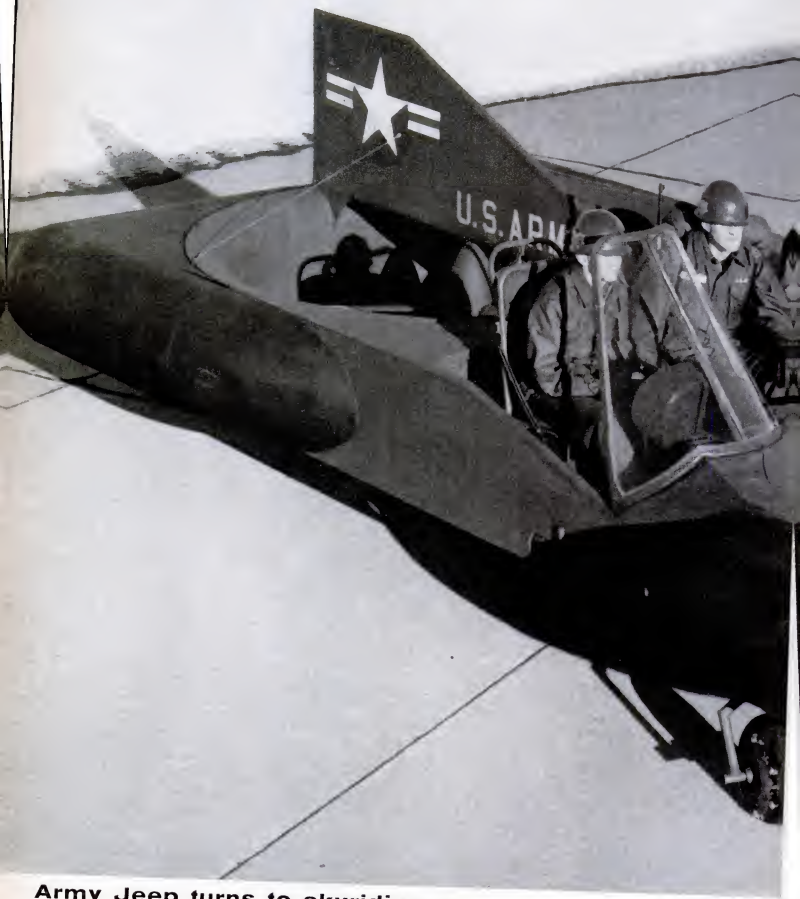
Army Jeep turns to skyriding. This new "Flying Jeep" will take off and land vertically, fly forward at 150 m.p.h. It is propelled by two rotors—one in front, one behind. It was developed as the 59K VTOL by Piasecki Aircraft Corp. for the Army as a high-utility, general-purpose
